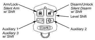
The Ungo MS2106 comes with 2 Random Code Remote Transmitters used to control the system's features. Each time a transmitter button is pressed, the LED will flash to indicate that a transmission is taking place.
